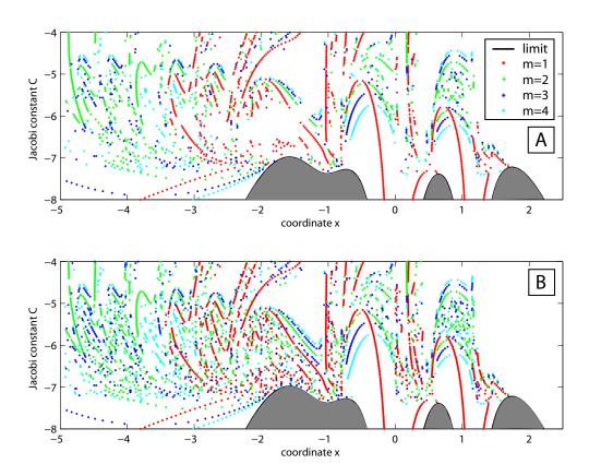
Figure 6: Symmetric periodic orbits (m denotes the multiplicity of the periodic orbit) in the most chaotic zone of the 7+2 Ring problem using double (A) and quadruple (B) precision. (Reproduced with permission from [23]).
