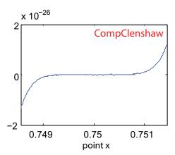
Figure 5: Evaluation of  $p(x) = (x - 0.75)^7 (x - 1)^{10}$  in the neighborhood of the multiple root x = 0.75, using Clenshaw (left) and Compensated Clenshaw (right). (Reproduced with permission from [60]).
