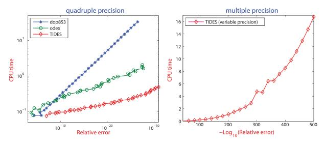
Figure 2: Left: Precision vs. CPU time diagram in quadruple precision for the numerical integration of the unstable periodic orbit LR for the Lorenz model using a Runge-Kutta code (dop853), an extrapolation code (odex) and a Taylor series method (TIDES). Right: Precision vs. CPU time diagram for the multiple-precision numerical integration of an unstable periodic orbit for the Lorenz model using the TIDES code.
