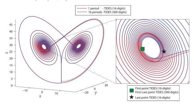
Figure 3: Numerical integration of the  $L^{25}R^{25}$  unstable periodic orbit for the Lorenz model during 16 time periods using the TIDES code with 300 digits and 1 time periods using double precision.
