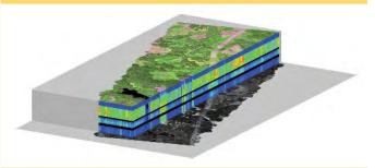
The data cube above was created from a hyperspectral image, which was taken by AVIRIS (Airborne Visible/Infrared Imaging Spectrometer) in 2002 over the Greater Victoria Watershed District. The image is 1988 pixels long by 1331 pixels wide, each pixel covering 4 metres on the ground.
