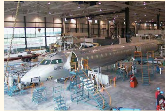
"Wingmating" – wing making in the Bombardier CRJ900
